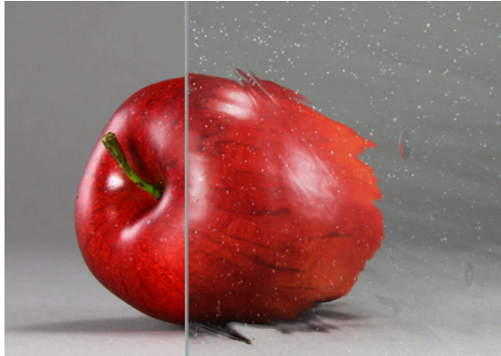
Fig. 1 - how seedy and reamy glass affect objects beyond a stained glass window
